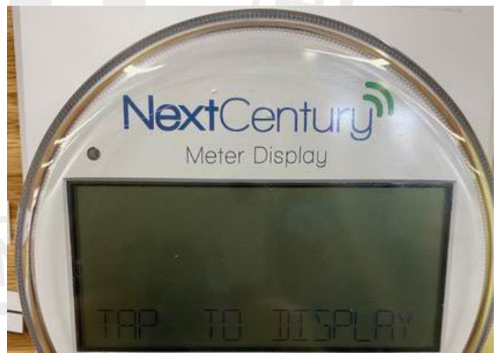
Figure 4. Example of the statement “TAP TO DISPLAY” mode. When this screen appears, one will need to tap the displace to activate the display.
