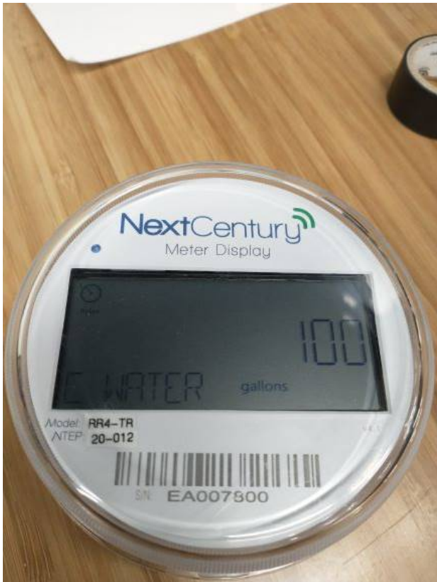
Figure 5. Example of the required ID markings on the face of the Model RR4-TR indicator with gallons
