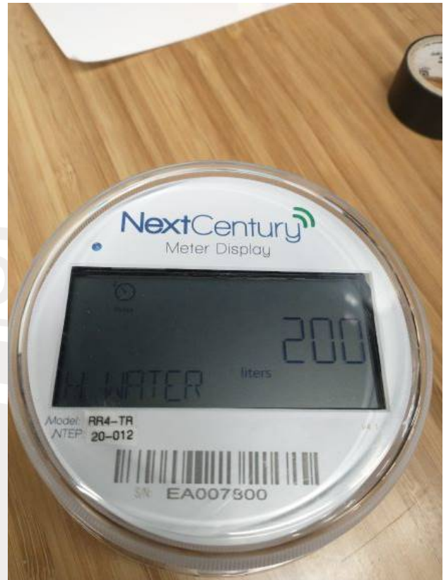
Figure 6. Example of the required ID markings on the face of the Model RR4-TR indicator with liters.
