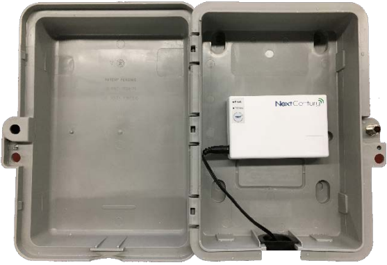
RE-201 inside NEMA Enclosure
