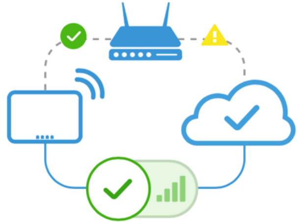
Figure 2 Gateway Connection Diagram showing a problem (alert icon) between the Router and NextCentury Cloud.
