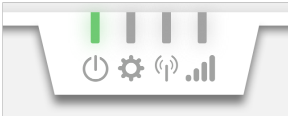
Figure 1 – LED Indicators on the GW-301. Powered on (green), but not connected to the NextCentury cloud (blue).
