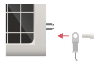
2) Attach the safety cable to the NextLink by removing one of the M8x18mm screws and using it to bolt the end of the safety cable to the mount bracket and NextLink.
