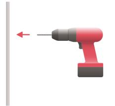
2) **Drill** the holes in the mounting surface using a **1/4" drill bit**.
