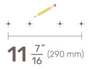
Drill the holes using a 1/4" drill bit.
