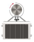
**Important**: Install the band clamps to no more than 18 inlbs of torque. Do not overtighten. Do not use an impact driver to tighten. Overtightening can compromise installation integrity.
