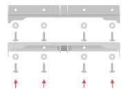
Attach the top of the NextLink to the top mount bracket using two (2) M8x18mm socket head cap screws. At this stage, these screws should be hand tightened.
