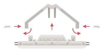
Attach one end of the pivot bar to the pole mount using the M8x50mm bolt and M8 locknut (see item **A** in the illustration below).
