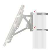
Fasten the band clamps around the pole. One person should hold the NextLink in place as the other tightens the band clamps around the pole.
