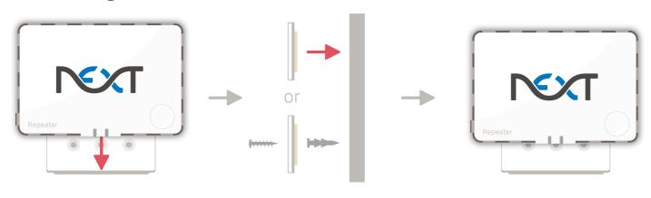
Remove the mounting plate from the Repeater
