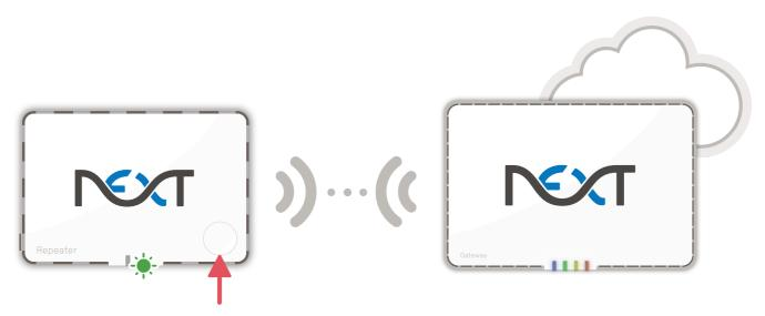
Press the Test Connect button to check the connection
