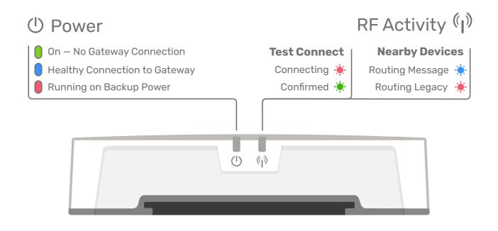
After pressing Test Connect, the RF Activity LED blinks slowly twice if the Gateway is reached. Fast blinks occur anytime signals are received from nearby devices.
